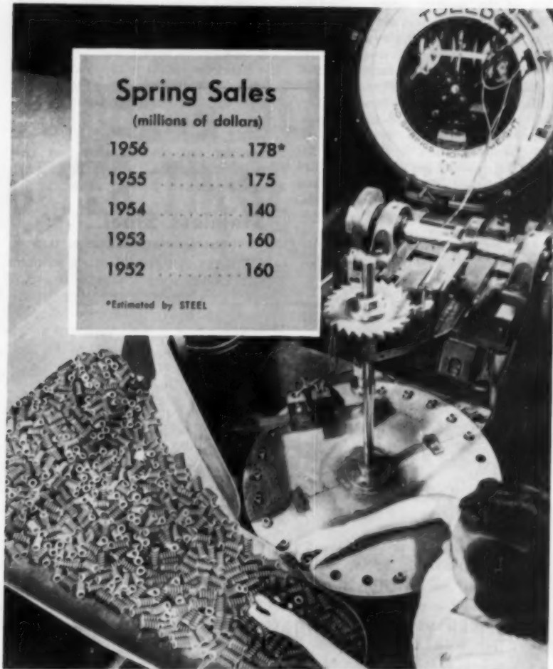
Compression springs are load tested for accuracy
